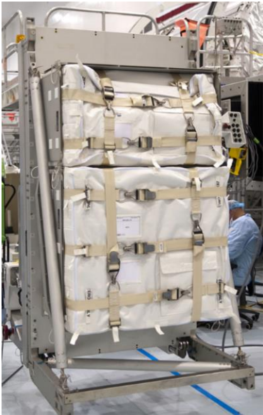
Resupply Stowage Platforms (RSPs) on the right with bags strapped in place.
