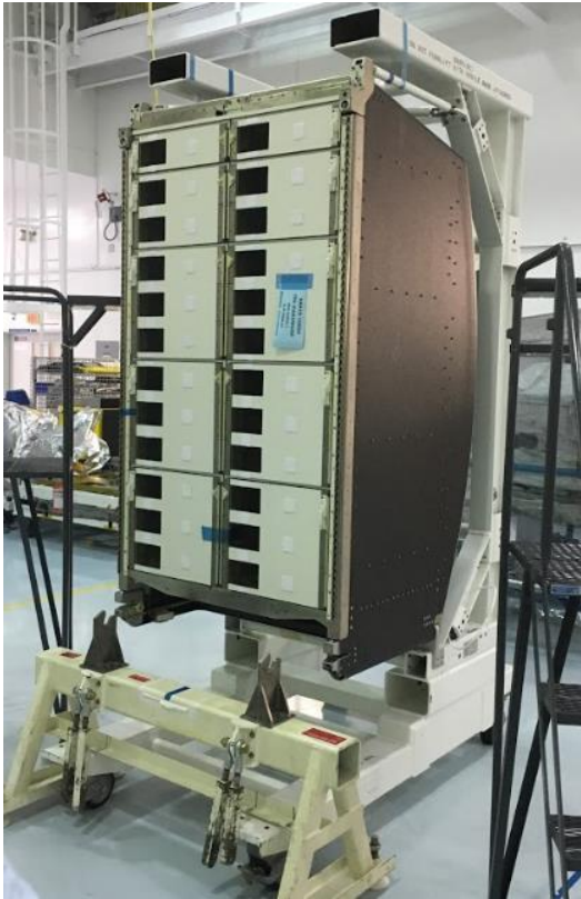
Resupply Stowage Rack (RSR) on the left with compartments and doors.
