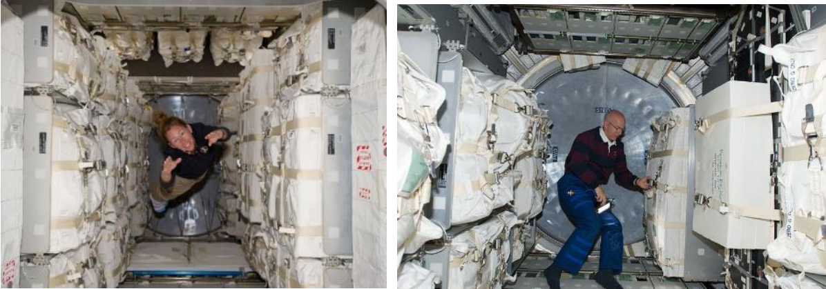
Resupply Storage Racks on sides. Resupply Storage Platforms on top and bottom.
