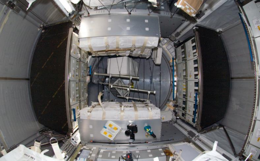
Resupply Storage Racks on sides. Resupply Storage Platforms on top and bottom.
